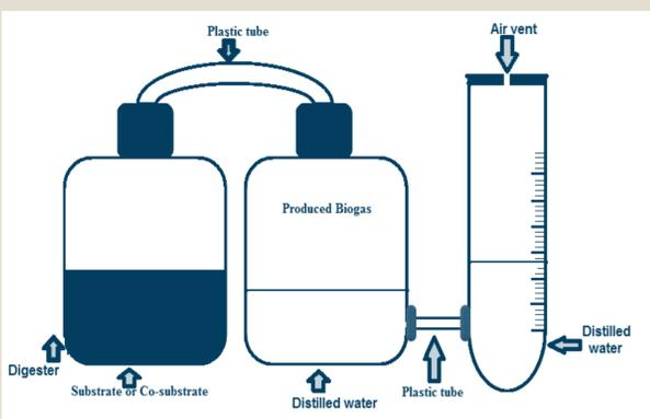
Figure 1. Laboratory Digester configuration
